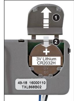
**Batterietausch / battery change**
