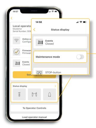
In the status display you can see all inputs and outputs of the operator and whether they are activated or deactivated.
