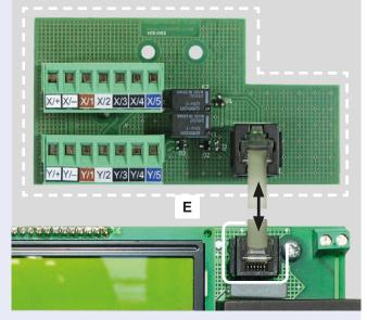
RJ-connection ST 64(A) with optional dropbolt module
