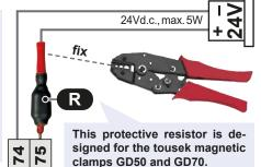
The magnetic clamps are used for the swing gate control units ST 51 and ST 61 for fixing the gate leaf in the open or closed position and for the barrier control unit ST 80 for locking the boom in the closed position.
