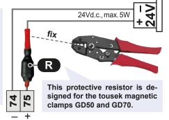
The magnetic clamps are used for the swing gate control units ST 51 and ST 61 for fixing the gate leaf in the open or closed position and for the barrier control unit ST 80 for locking the boom in the closed position.
