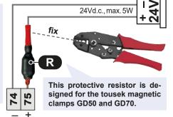
The magnetic clamps are used for the swing gate control units ST 51 and ST 61 for fixing the gate leaf in the open or closed position and for the barrier control unit ST 80 for locking the boom in the closed position.
