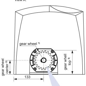
Fixing of the gear wheel: - PULL T4, T5, T8, T10: Seeger ring - PULL T15: with screw
