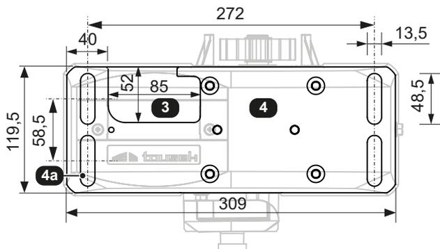
**PULL T15: depth of ground plate = 12mm**
