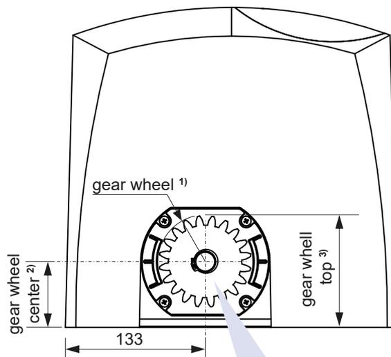
Fixing of the gear wheel:
