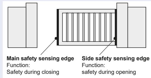
Hence if safety edges have to react on obstacles in closing movement have to be serially connected to the terminals of the main safety edge.
